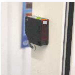
PEC mounted on the guide section
